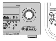
Adjust the volume to a comfortable level using the **VOLUME** control knob on the front panel or the **VOL**  $\triangle$  /  $\nabla$  buttons on the remote control unit. To increase the volume, turn the **VOLUME** knob
